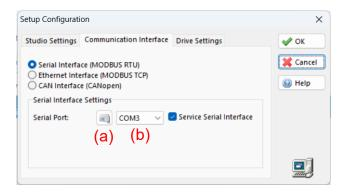
In case you have a drive that has the connection for a Service Serial (one out of the three cables shown previously), then select the first communication interface in this window. Now check the ports number that are available (a). Select one of the available ports here (b). Click **ok**.
