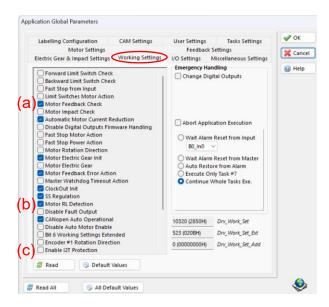
If you want to work in closed loop, select the option *Motor Feedback Check* (a). If you want to read the Inductance and resistance of the motor, select the *Motor RL Detection* (b). Set the flag *Enable I2T Protection* (c) to have a protection from high currents.
