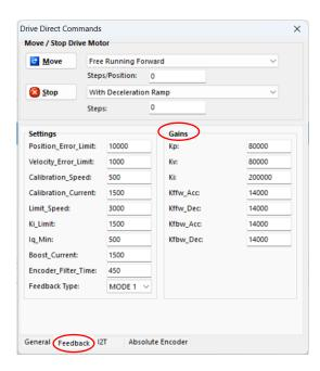
In the same window, you can tune the gains of the control, Kp, Kv and Ki. If you are working with a stepper motor it is better to put lower values of the gains with respect to the default ones. For example, try with Kp=1000, Kv=Ki=25000.
