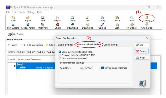
Depending on the communication interface that you are using, you have some parameters to set (e.g. Serial port and Baud Rate, IP Address and port, CAN Board, Address and Rate). In the following picture you can find the three possibilities with the default values for each case.
