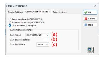
In case you have a drive based on CAN or an integrated motor that does not have the connection for the Serial Interface, then you need a CAN converter, it can be for example: GCAN (property of Delta-Line), IXXAT, PEAK.
