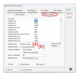
Scroll the parameters until you find **Feedback\_Boost\_Current**() and set the value of the peak current that is written in the datasheet of your motor.
